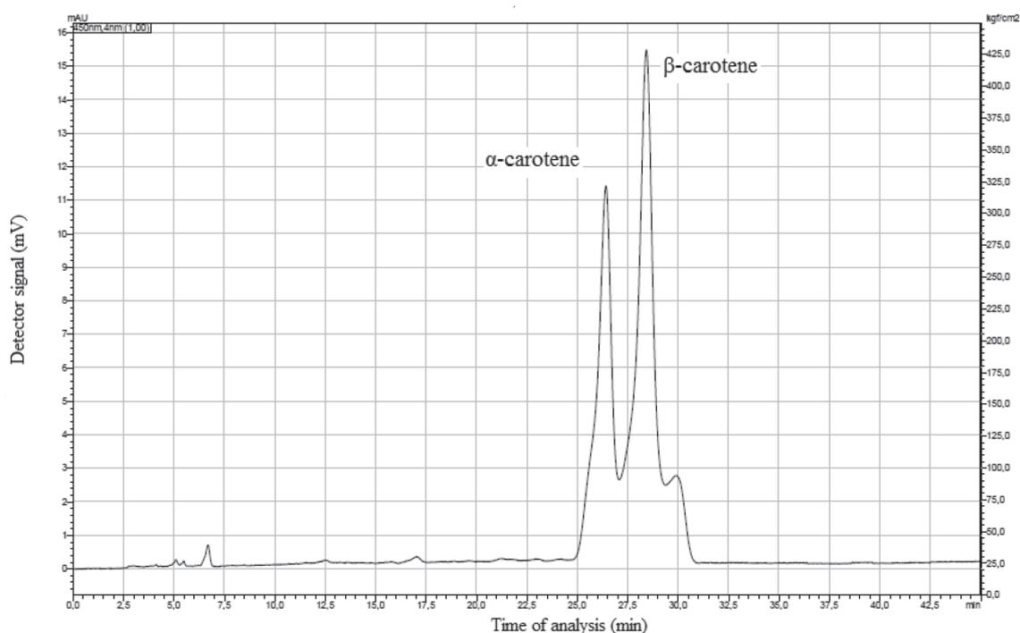
FIGURE 1. Chromatographic separation of  $\alpha$ - and  $\beta$ -carotene, detection at  $\lambda = 450$  nm.
